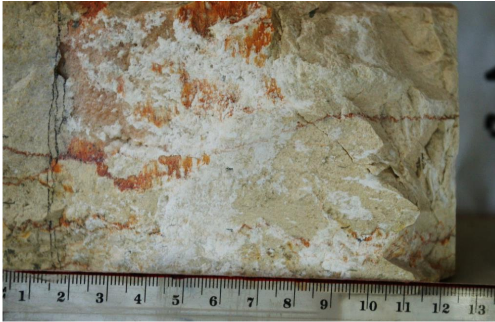
Figure 4.37. Post-shear photograph of sample LN5, bottom surface. The damage zone is visible in the right-hand side of the surface, note the jagged formations of broken rock when viewed from above. More damage and welded wear is visible on the rest of the surface in the white patches.
