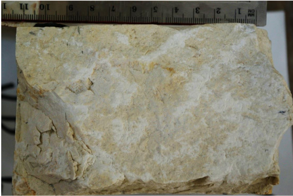
Figure 4.31. Post-shear photograph of sample LN6, bottom surface. The damage zone is seen on the bottom-left corner of the surface. The zone appears as a “hole” in the surface and includes tilted fractures dipping to the left. Shear direction is to the left-hand side of the picture.
