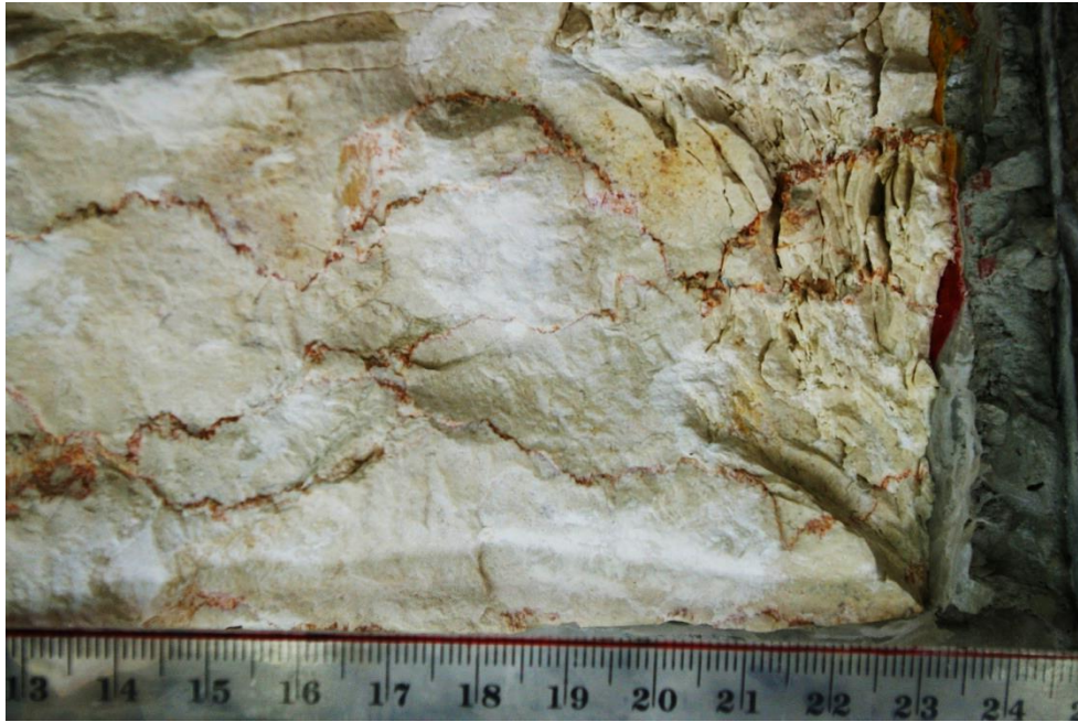
Figure 4.28. Post-shear photograph of sample LN10, top surface. The damage zone is visible on the right-hand side of the picture; it includes many tilted fractures, dipping to the right, and small white patches of pulverized rock. Undamaged zones can be seen to the left of the picture where the rock looks “fresh”. The areas covered in white powder are the welded wear localities. Direction of shear is to the right-hand side of the picture.
