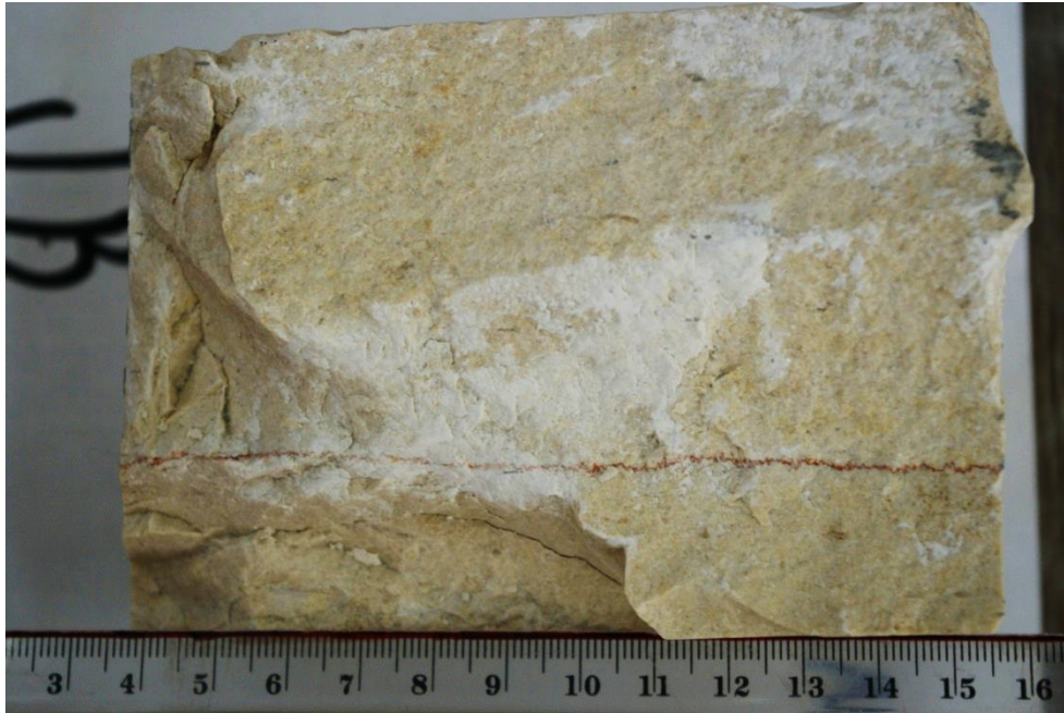
Figure 4.40. Post-shear photograph of sample LN7, bottom surface. The damage zone is seen to the bottom-left corner of the surface. Notice the small fractures in the central white patch, their dip and direction is similar to the fractures in the damage zone.
