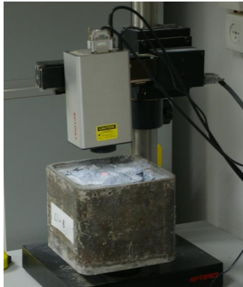
Figure 3.5. The laser profilometer at Geological Survey of Israel during a surface scan. Note that the surface is scanned while still in the steel frame which helps adjust the pre and post-shear scans in the same scanning orientation.
