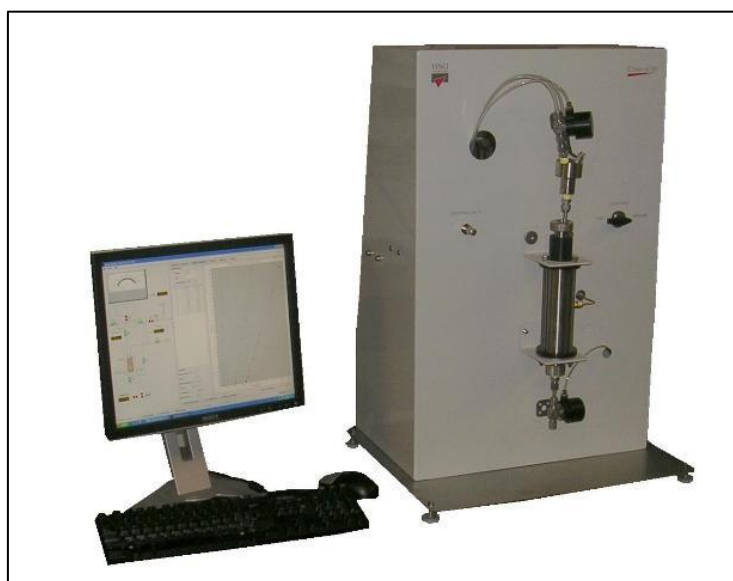
Figure 16: The Coreval 30 permeameter and porosity meter manufactured by Vinci technologies (photo from www.vinci-technologies.com ).
