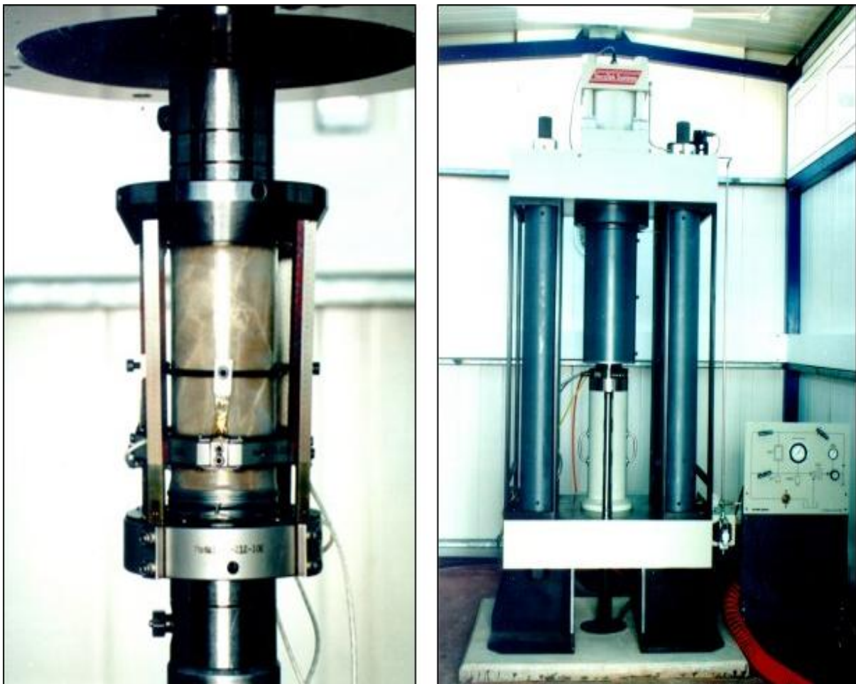
Figure 9: To the right, 1.4 MN stiff load frame and 70 MPa confining pressure vessel located at the Rock Mechanics Laboratory of the Negev. To the left, the four arm radial and axial strain cantilever gauge system.
