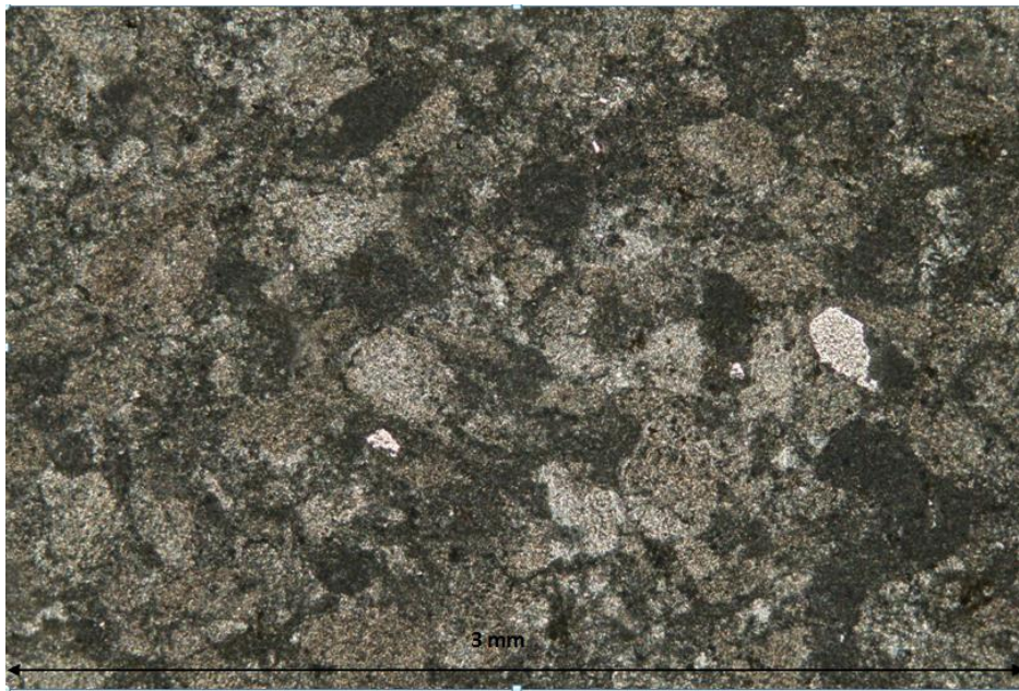
Figure 18: An example of a thin section of the tested limestone.
