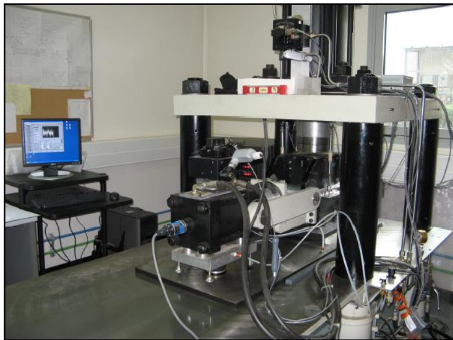
Figure 6: A general view of the direct shear system DS-4250 at Rock Mechanics Laboratory of the Negev at Ben-Gurion University
