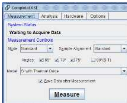
Figure 4-9. To measure the Reference Wafer, select “Standard” Mode, “Standard” Sample Alignment, all three Off-Sample Angles (65°, 70°, and 75°). The Model for the Reference sample is “Si with Thermal Oxide” found in the Basic Folder.
