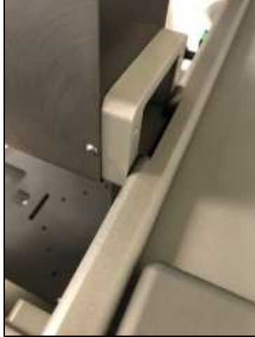
Figure 7-8. Align Camera Mounting Plate with Z-Stage Post.
