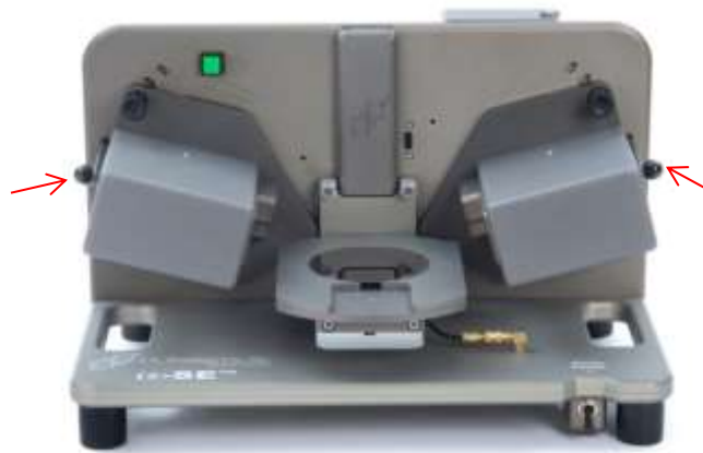
Figure 4-2. Support knobs for lifting the Source and Detector when changing the Angle of Incidence.
