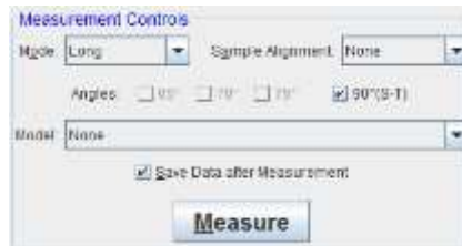
Figure 4-7. Settings to test Straight-Through Accuracy of ellipsometer, measuring air.
