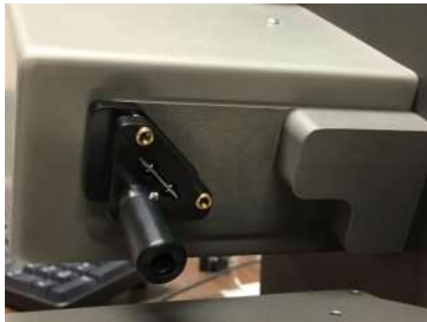
Figure 7-2. Source probe installed.
