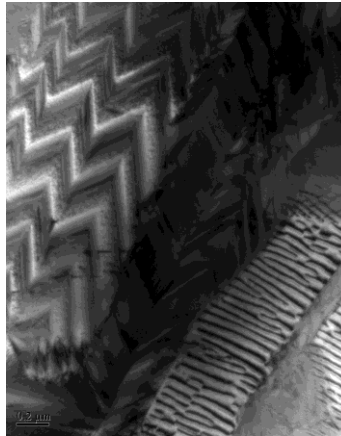
Fig. 2. Alternating sequence of \sim 200\text{nm} of GeTe and PbTe rich phases, containing submicron twinning and dislocations, respectively, for \text{Ge}_{0.5}\text{Sn}_{0.25}\text{Pb}_{0.25}\text{Te} .
