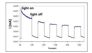
Photovoltaic current in nano-structured photoelectrochemical cell
