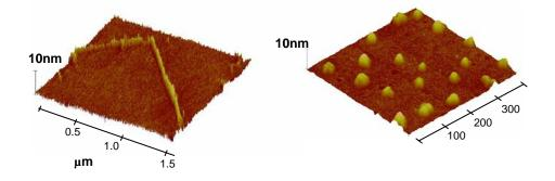
Figure 2: gold nanostructures created via diacetylene monolayers.
