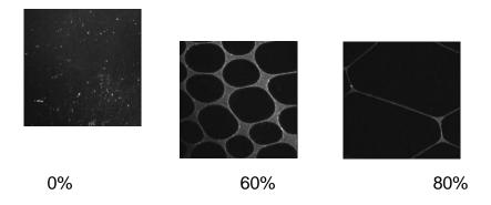
**Figure 3: BAM images of Au-NP/elaidic acid Langmuir monolayers at different laser intensities.** The percentage values indicate laser power used for monolayer irradiation prior to image acquisition:
