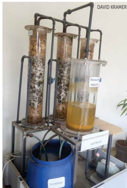
A DEVICE DEVELOPED AT BEN-GURION UNIVERSITY distills nitrogen from manure to produce liquid fertilizer that can be applied by drip irrigation. The university is seeking funding to scale up and commercialize the process.
