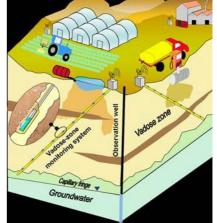
very shallow soil depths. This limitation has led to the development of a new Vadose zone Sampling Port (VSP) apparatus that is based on structural modification of tensiometers and a special installation technique that allows installation of multiple probes all along the deep vadose zone cross-section from land surface to groundwater. Using this VSP system enables easy, continues monitoring of a pollution process.
