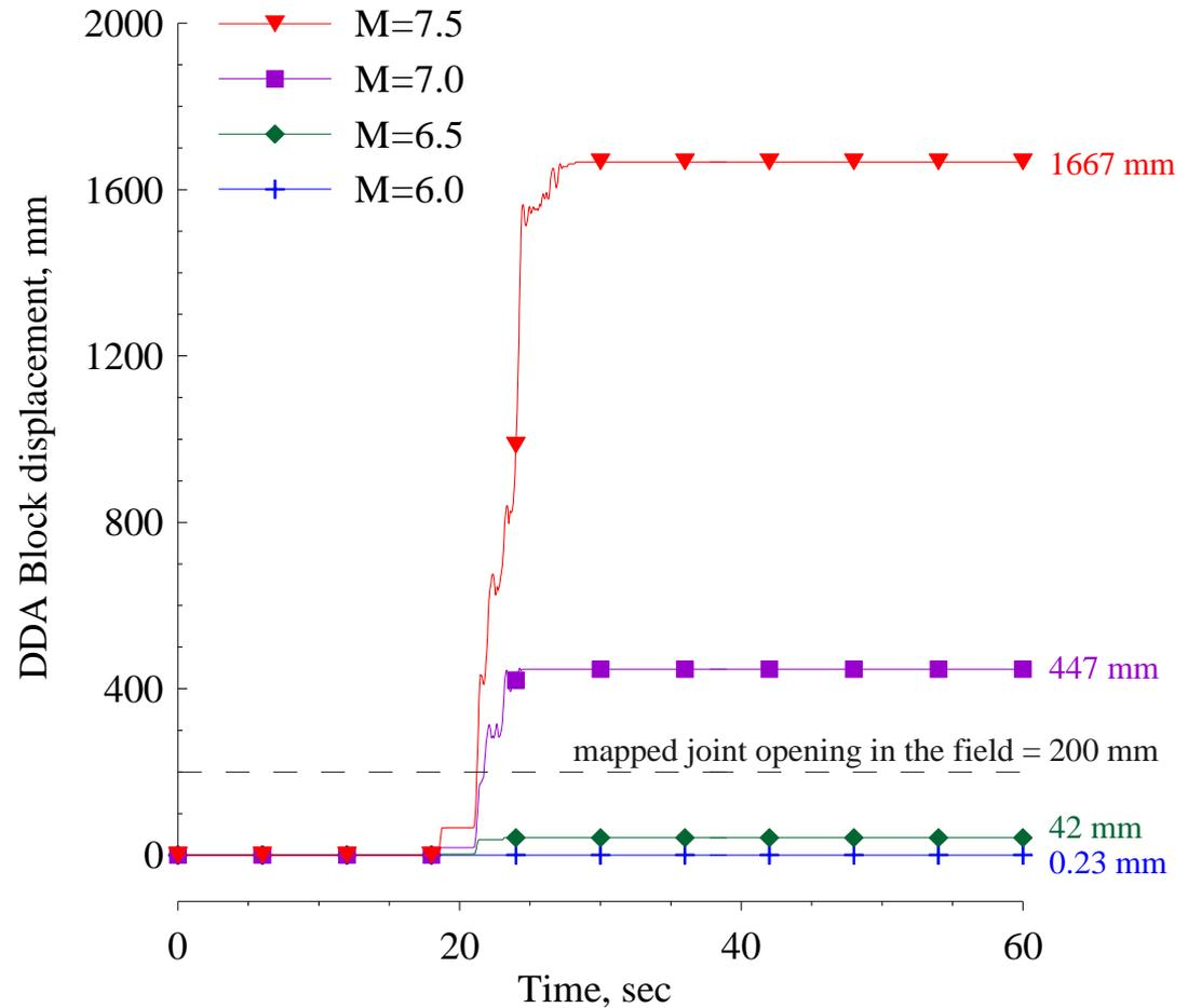
DDA results for dynamic displacement of Block 1 when subjected to amplified Nuweiba records corresponding to earthquakes with moment magnitude between 6.0 to 7.5 and epicenter distance of 1 km from Masada. Mapped joint opening in the field is plotted (dashed) for reference.
