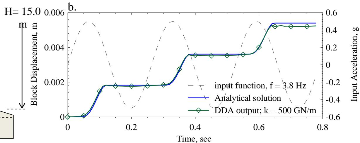
DDA results are strongly affected by the penalty, or contact spring stiffness, value, especially in dynamic simulations. We optimize the contact spring value using the analytical (Newmark) solution and the two measured resonance frequency modes of the mountain: 1.3 Hz and 3.8 Hz.
