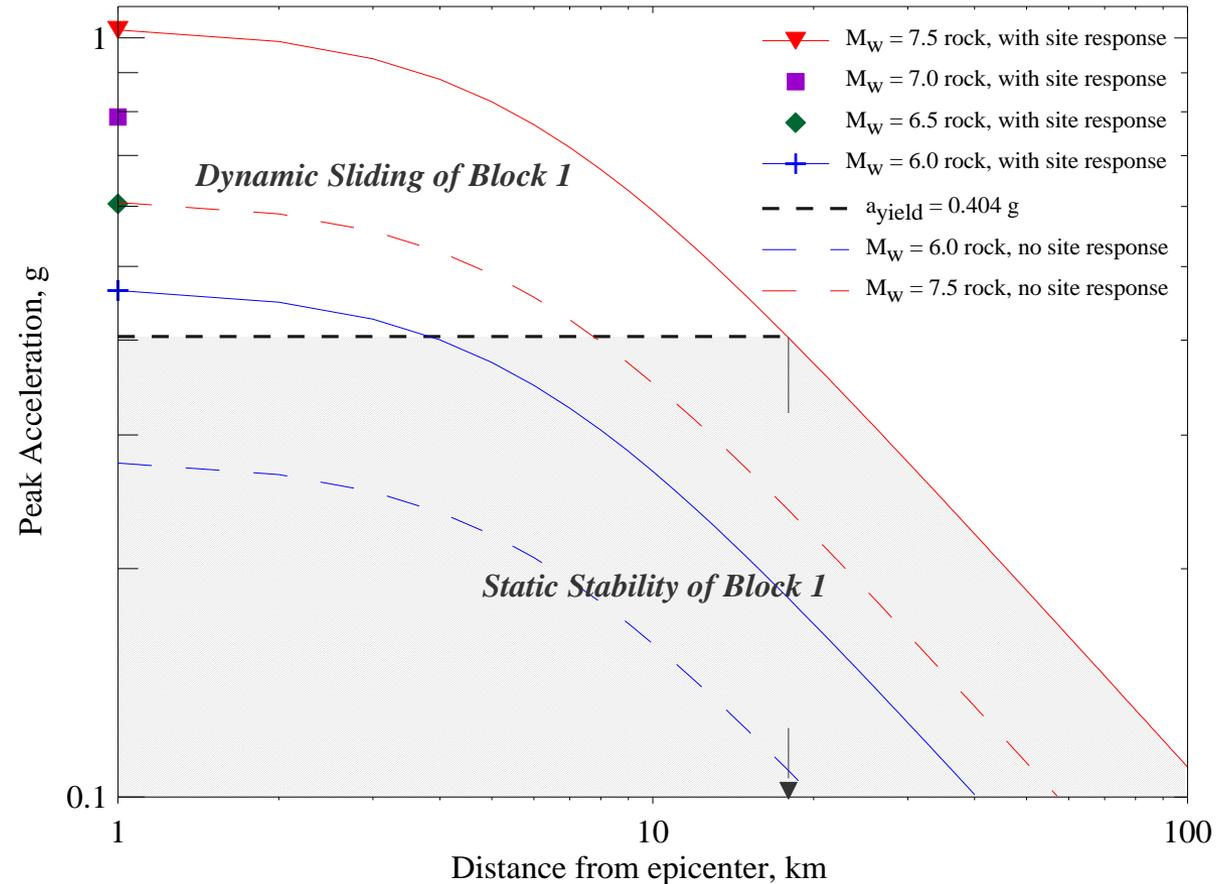
Assumed attenuation curves for Dead Sea Rift earthquakes [after Boore et al., 1997] (dashed lines) with amplification due to topographic site effect at Masada (solid lines and symbols). Shaded region delineates conditions at which seismically-induced sliding of Block 1 at Masada is not possible.
