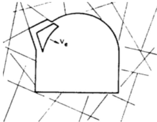
Figure 6.1 Ejection-type rockburst results from expulsion of joint or fracture-defined block of rock. (Ortlepp & Stacey ,1994)
