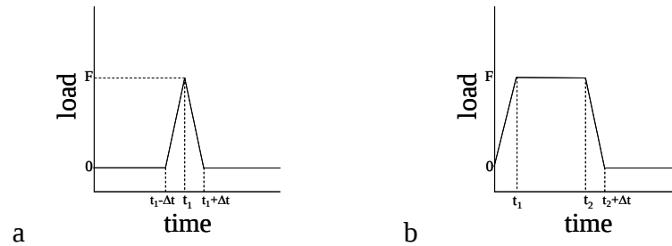
Figure 3.7: Input loading functions used as input in 2D-DDA simulations: a) dynamic load function used to simulate sledgehammer impulse applied at the base of the column, b) static load function used to simulate the push and release applied manually at the top of the column.
