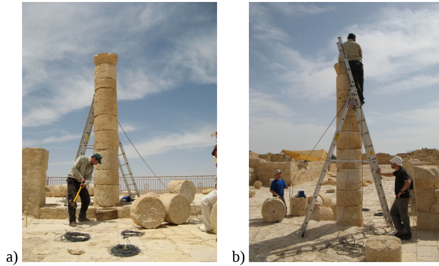
Figure 3.5. Different excitation modes at the experimental site response survey. a) sledgehammer blows to the bottom of the column and b) manual push to the top of the column.
