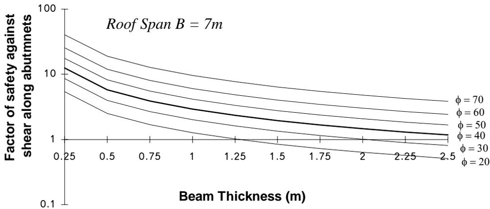
Figure 4. Sensitivity of factor of safety against shear sliding along the abutments to the available friction angle and to the beam thickness according to classic voussoir beam analysis
