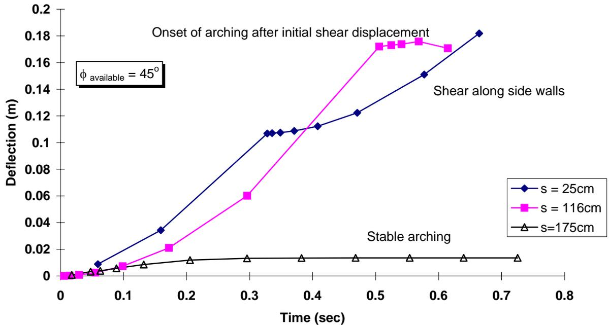
Figure 9. Three different “Beam Reaction Curves” for three different voussoir beam configurations as predicted by DDA.
