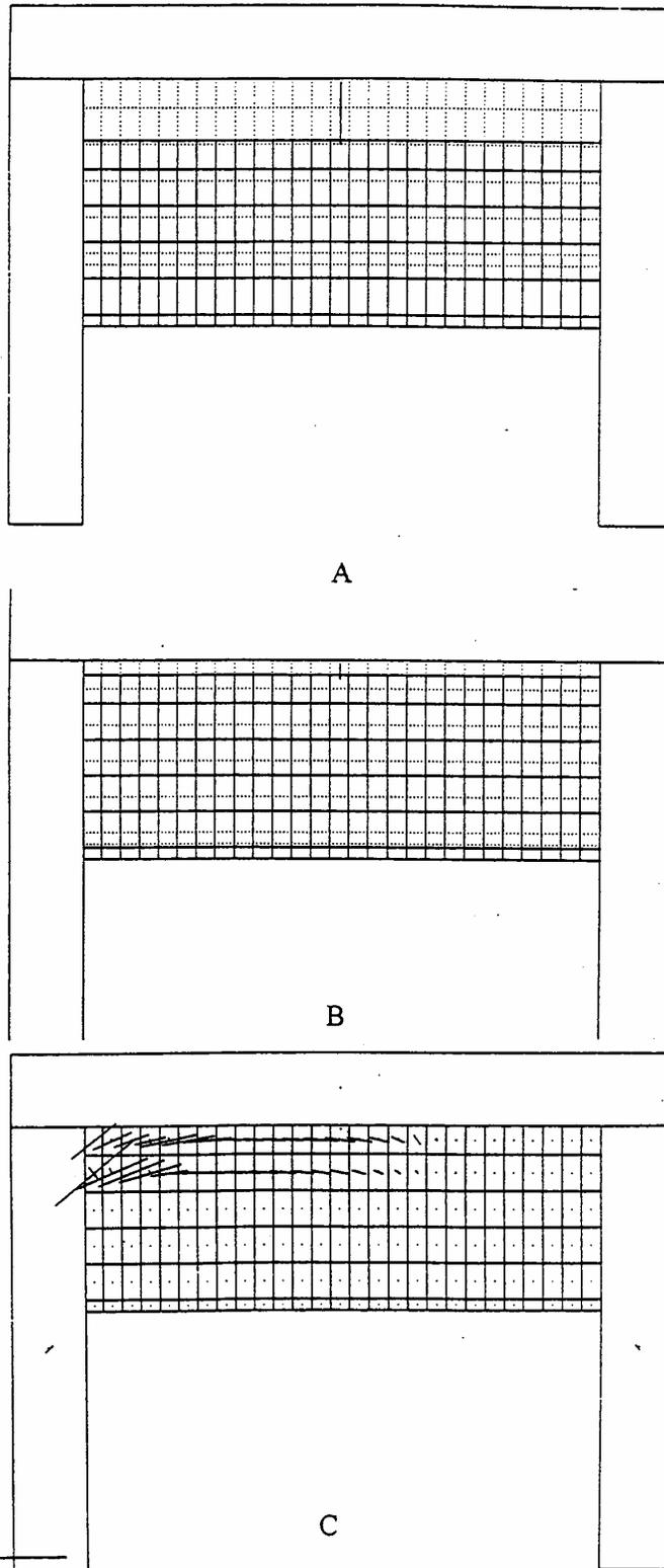
Figure 5. Three DDA experiments for the deformation of a laminated Voussoir beam after 25 time steps (see text for details). Beam geometry:  $B=7\text{m}$ ,  $d=2.5\text{m}$ ,  $t=0.5\text{m}$ ,  $s=0.25\text{m}$ . A)  $\phi_{\text{available}}=20^\circ$ ,  $u_{\text{max}} = 0.83\text{m}$ ; B)  $\phi_{\text{available}}=40^\circ$ ,  $u_{\text{max}}=0.2\text{m}$ ; C)  $\phi_{\text{available}}=85^\circ$ ,  $u_{\text{max}}=0\text{m}$ .
