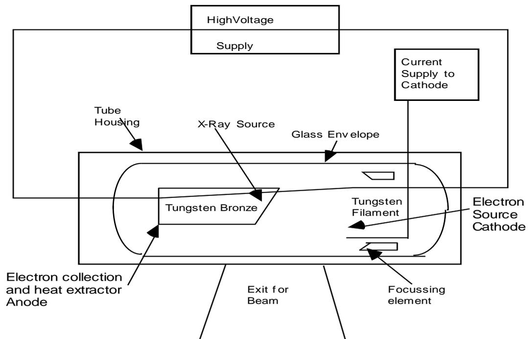
**Target:** The electrons bombard a target made of tungsten. Since only part of the electron energy is converted into X-radiation, much heat is created in the target, and so a suitable means of cooling it must be supplied. The proportion of electron energy converted into X-radiation is relatively low. An approximate equation gives  $10^{-3} \times$  atomic weight of the target  $\times$  electron energy = X-radiation energy
