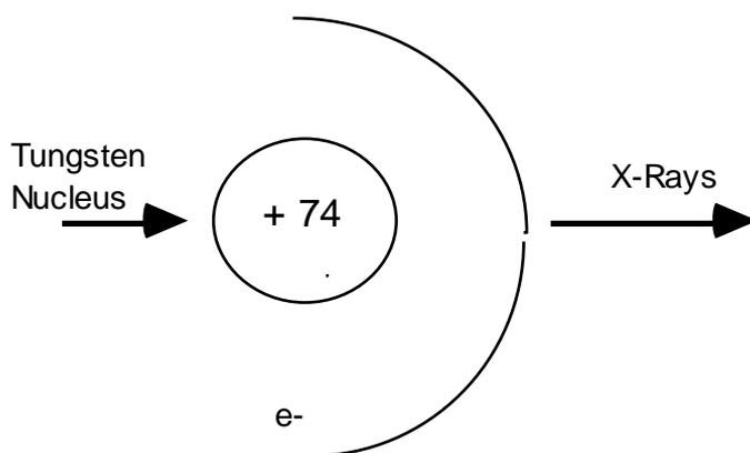
In Figure 1 we see an accelerated electron approach the electric field of a heavy nucleus such as tungsten (with 74 protons). As a result, the electron is slowed and changes its direction, i.e., loses energy. This energy is emitted as X–radiation
