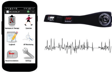
Figure 2. The MobiGuide app; ECG sensor with chest belt, and an atrial fibrillation event detected by the ECG sensor.
