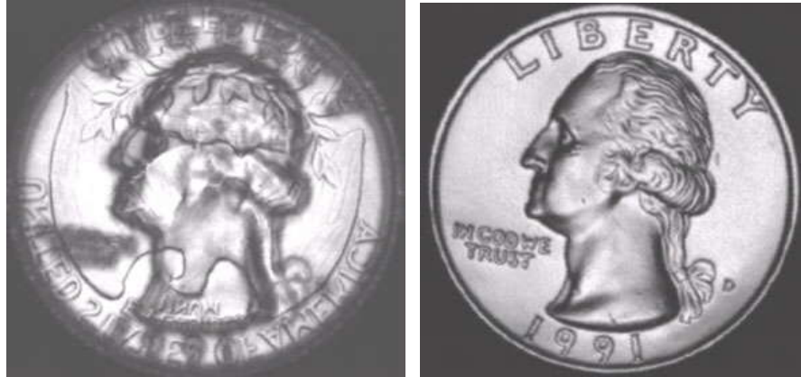
figure 27: ultrasonic C-scan images of a US quarter
