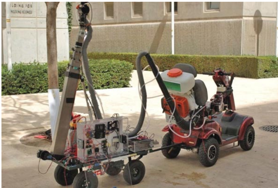
Figure 1. The 1:6 scaled-down prototype in a folded configuration.
