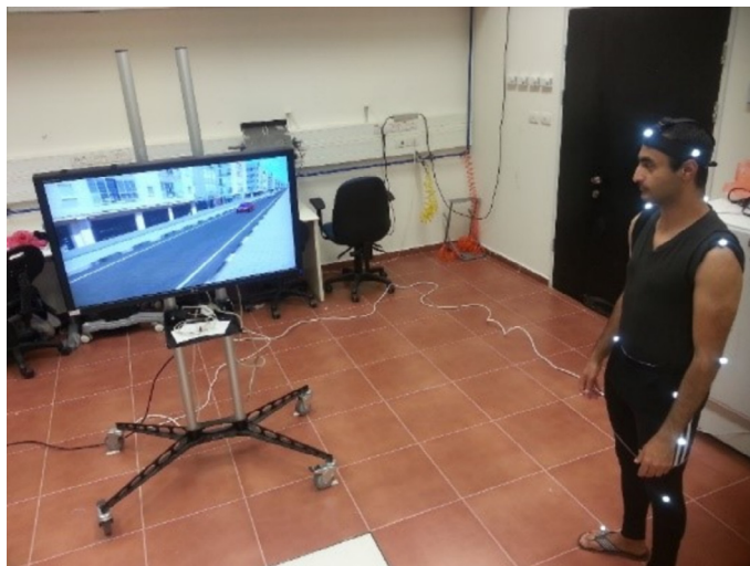
Fig. 1. The experimental setup. A participant looking at a simulated crossing scenario where traffic is approaching from the right.
