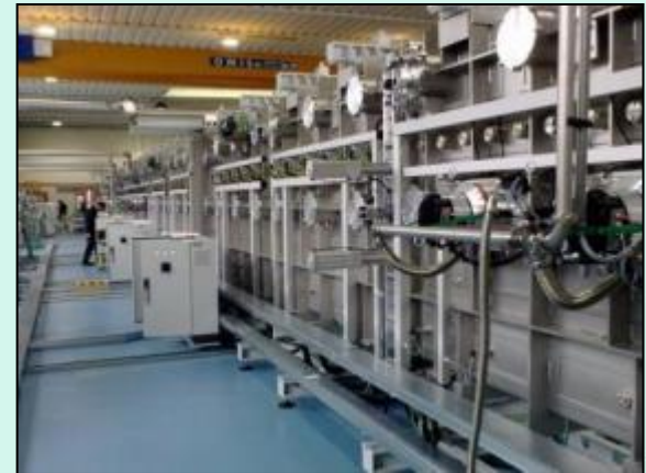
Industrial sputtering apparatus to fabricate ENEA solar coating at the manufacturing site - Massa Martana (PG, Italy)
