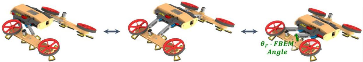
Figure 3.4 - Definition of the FBEM angle. By changing the FBEM angle the width and the length of the robot can be changed.
