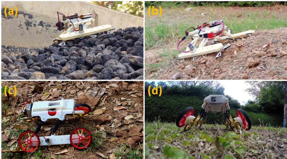
Figure 5.1 – RSTAR crawling on variety of surfaces including gravel, soft ground, leaves and grass (see video [24]).
