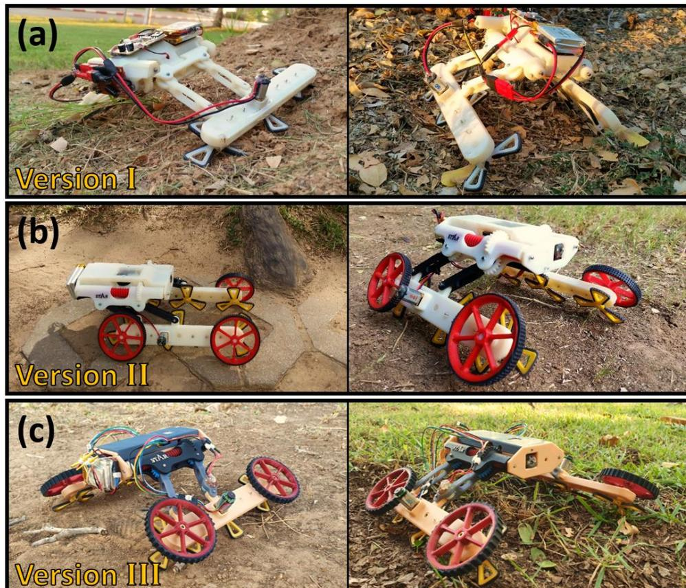
Figure 3.8 – The three versions of the RSTAR produced through this research.
