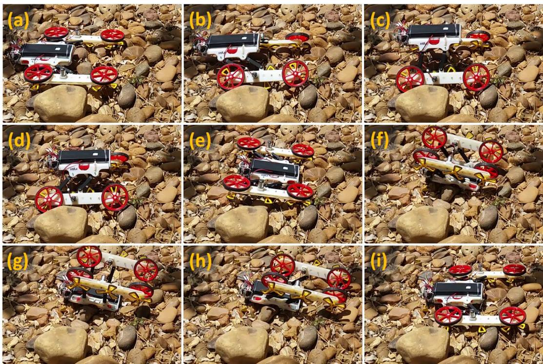
Figure 5.3 – Full cycle of turtle gait locomotion, the RSTAR is advancing forward using its legs without rotating its wheels (see video [24]).
