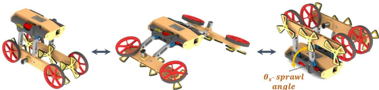
Figure 3.2 – Definition of the sprawl angle, the relative angle between the legs and the main body. Changing the sprawl angle can increase or lower the robot width and height.
