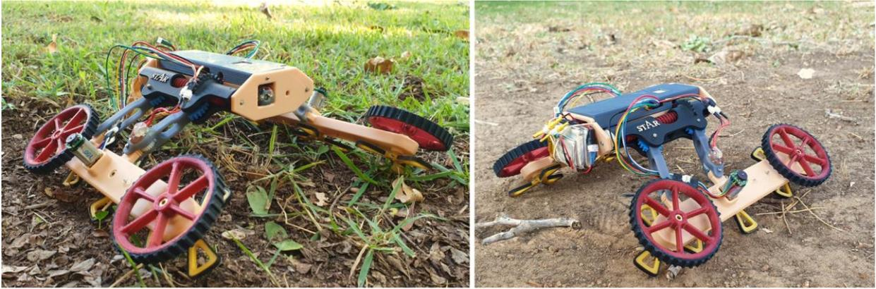
**Figure 1.1 - The Rising STAR (RSTAR) robot is a highly reconfigurable robot for search and rescue proposes (see video [24]). The sprawl mechanism allows the robot to move in and out of the plane whereas the four bar extension mechanism (FBEM) extends the arms holding the legs and relocates the center of mass.**
