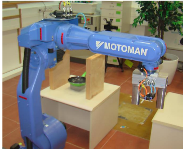
Figure 30 – Motoman UP6 Manipulator used for validation in hardware
