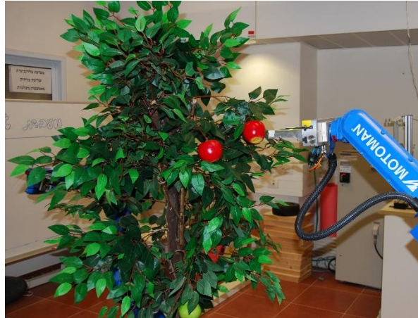
Figure 2 – Robotic arm picking an apple at the Tele-robotics lab at Ben Gurion University
