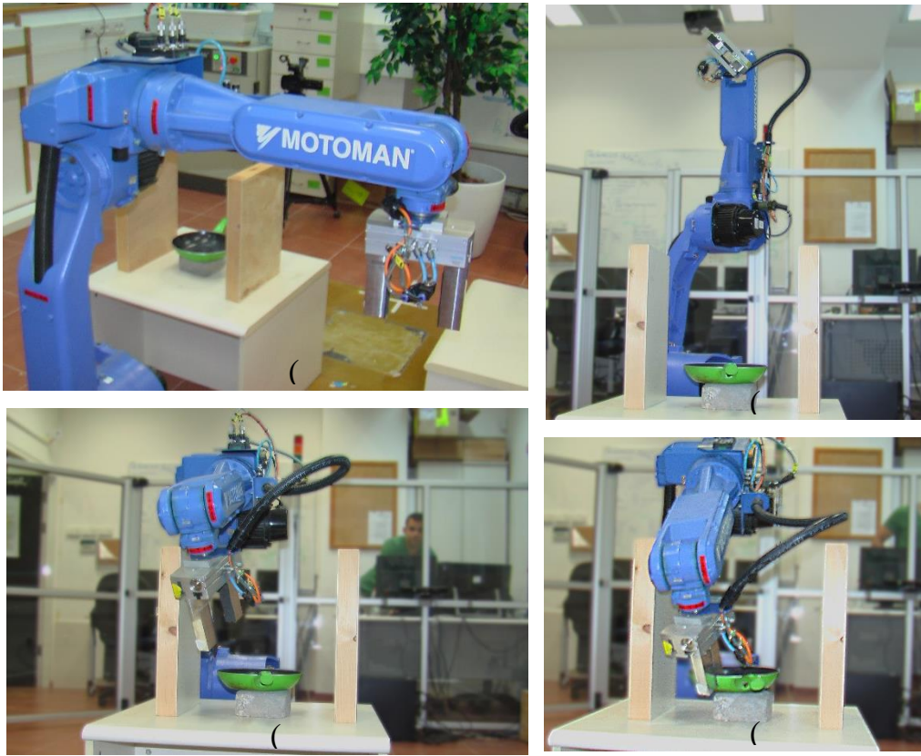
Figure 32 – Illustration of reach-to-grasp of a pan with the UP6 manipulator (a-b) initial position, (c) the offset pose relative to the final grasp, (d) final grasp.
