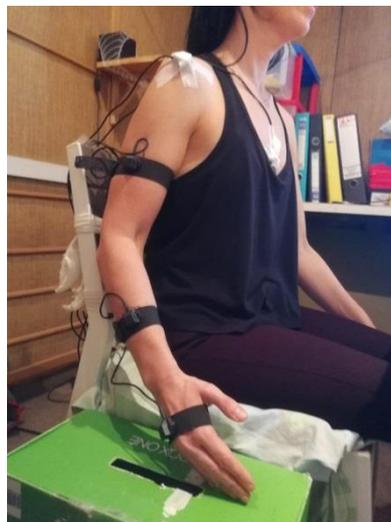
**Figure 5** : Sensors positions. Movement was recorded using 5 sensors, each measuring 6 degrees of freedom with respect to a base calibration frame and is tracked at 120Hz. Sensors were placed on the midsternum, midpoint of the acromial superior-lateral border, midpoint of the ventrolateral arm, dorsal forearm (1/3 forearm length proximal to ulnar head), and the index metacarpophalangeal joint.
