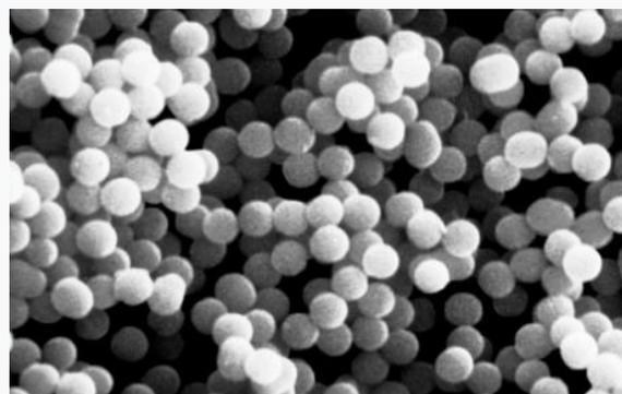
**Picture 1.** Encapsulation scheme of amphiphilic material in the proteinoid capsule and an SEM image of the nanocapsules
