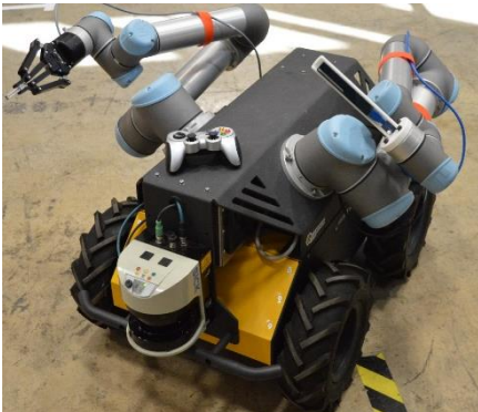
The VaultBot dual-arm mobile system (left) under the control of a USW (United Steel Worker) union operator using UT's hands-free, voice recognition interface (center) and a mobile inventory/inspection/survey vehicle with its new operators and employees of the Portsmouth Gaseous Diffusion Plant (right).
