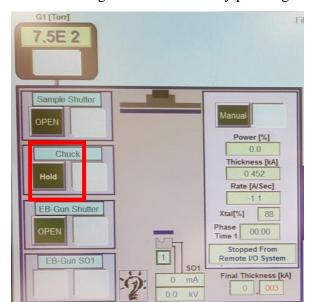
10. Load the stage to the chamber by pressing chuck "hold" button.
