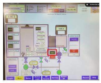
9. Insert the stage inside the main chamber with the arm. Check that the arm status is changed from "arm outside" to "arm inside".
