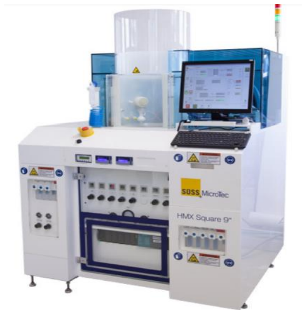
HMX Square Machine: Strip / Clean + Develop + Etch Photomask Processing
