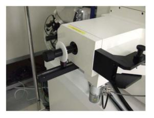
When the load lock vacuum is ready, open the load lock valve, insert the rod and click OK
