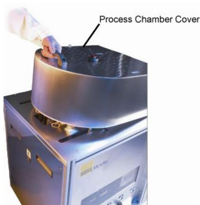
**Figure 6-1 Process Chamber Cover**
