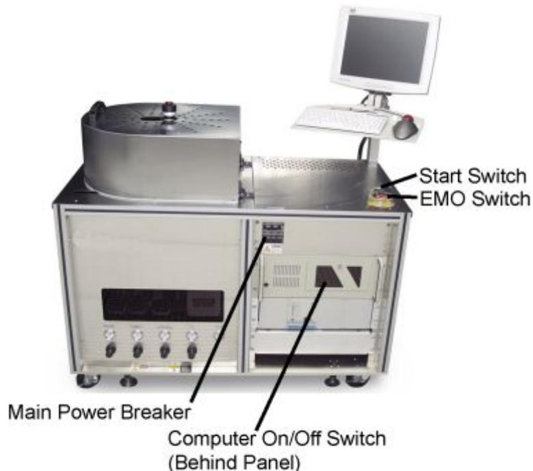
**Figure 6-5 Location of Equipment Power Switches**
