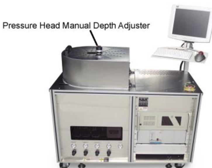
Figure 5-19 Location of Pressure Head Manual Depth Adjuster
