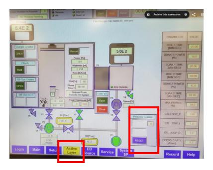
10. When the power start to increase wait for the crucible to be red (to have melting) and then make sure that the beam is at the right position.
