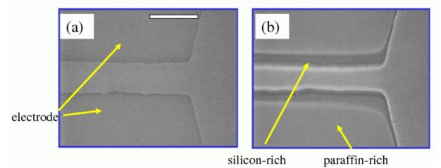
Field-induced phase transition in mixtures of simple liquids. (a) Field off. Two flat electrodes are covered with homogeneous mixture of silicon oil and paraffin. (b) Field on. Silicon-rich domains form close to the electrodes' edges, paraffin-rich phase is elsewhere. Bar is 50  $\mu$ m [*Nature* **430**, 544 (2004)].
