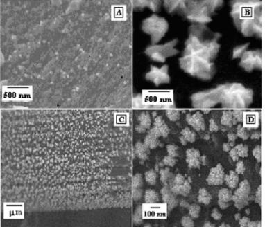
SEM cross section micrographs for particles of: Pd (A), Au (B) and Au-Pd alloy (C)&(D), embedded in cross linked poly(4-vinylpyridine) and incorporated in aerogel carbon.
