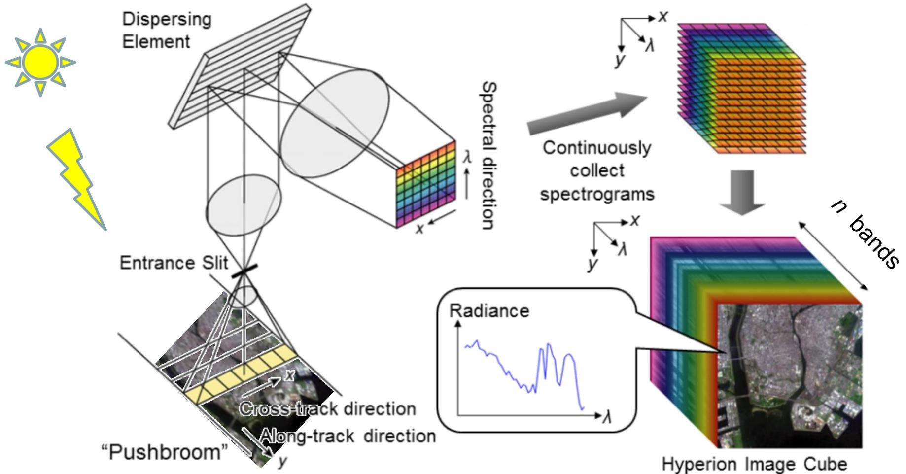
Figure 1. Hyperspectral imaging
