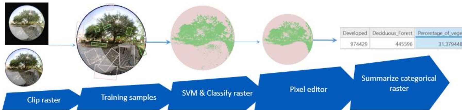
Figure 2 – the process of computing the percentage of vegetation from fisheye pictures in ArcGIS PRO.
