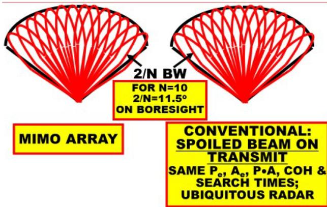
**Figure 5** MIMO monostatic linear full array of  $N$  elements and its conventional equivalent using spoiled beam on transmit, Ubiquitous radar; volume FOV search of  $120^\circ$ .
