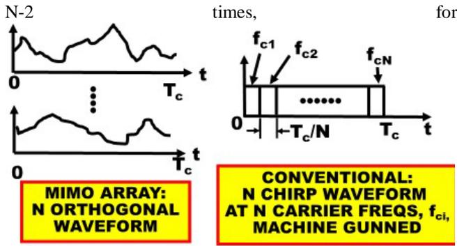
**Figure 4.** Waveforms for MIMO thin/full array & conventional equivalent.
