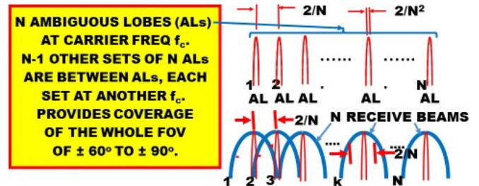
Figure 3. Conventional thin/full linear array; thin on transmit, full on receive;  $N$  elements each.
