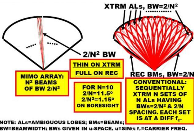
Figure 2. MIMO thin/full array & conventional equivalent; thin on transmit, full on receive; each  $N$  element linear array; volume search of  $120^\circ$ .
