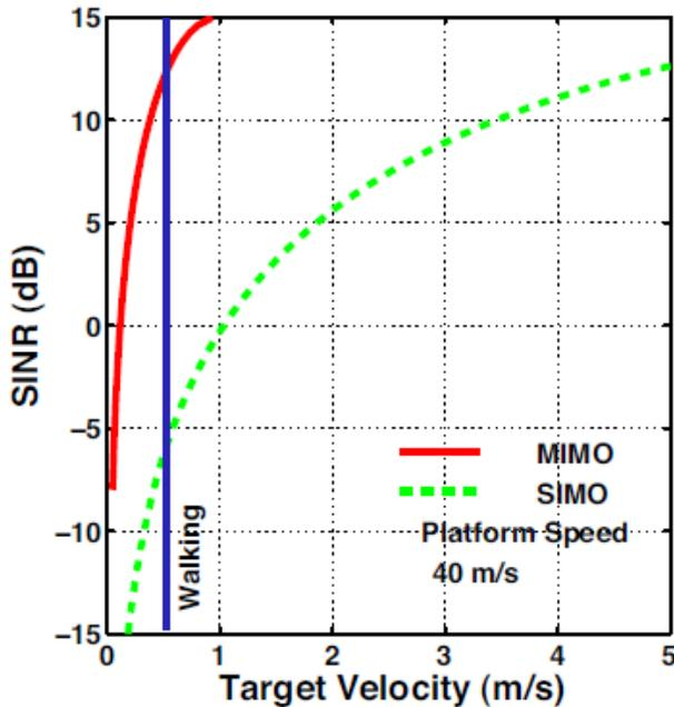
**Figure 6.** Comparison of MIMO and conventional GMTI systems. Assumptions: MIMO: thin/full array,  $N=5$ ; Conventional: full array,  $N=5$ . From [28].
