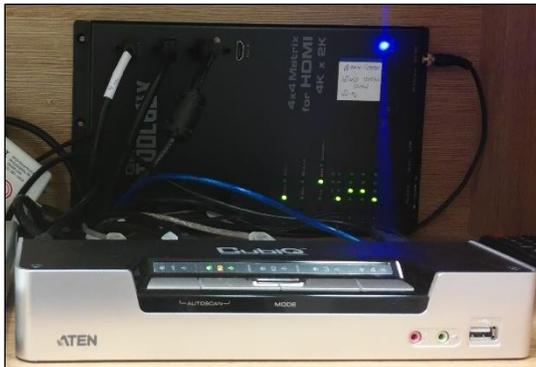
2. **GEFEN Toolbox** - Used to switch screen to the subject. The device is connected to the three screens - old, new, and TV. This device sets the output screen by pressing the desired screen number repeatedly. For example, if we use the number 2 computer with the old screen, we will set Output 2 and Output 3 to Input 2 - as shown in the picture.
