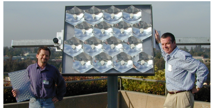
Figure 3. Prototype modules of Generations 1 (right, on a two-axis solar tracker) and 2 (left).
