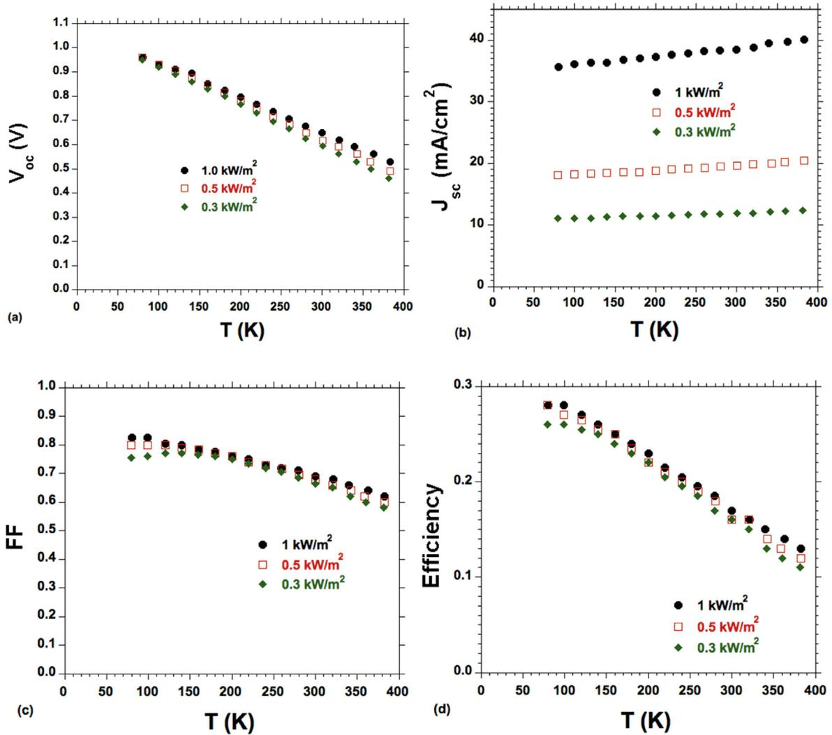
**Fig. 2.** Representative measured PV performance variables plotted as a function of  $T$  from 80 to 380 K, at irradiance values of 0.3, 0.5 and 1.0  $\text{kW/m}^2$ . (a)  $V_{oc}$ . (b)  $J_{sc}$ . (c) FF. (d)  $\eta$ . The experimental uncertainties (error bars) for  $V_{oc}$ ,  $J_{sc}$ , FF and  $T$  are smaller than the symbols indicating the data points, and are  $\pm 5\%$  relative for  $\eta$  based on the accuracy for measuring irradiance.
