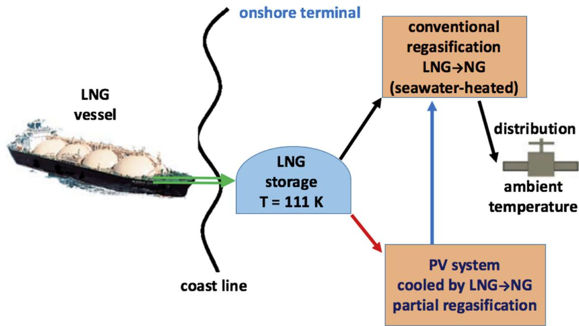
**Fig. 1.** Schematic indicating that part of the LNG received and stored at an onshore terminal can cool an on-site PV system. Natural gas exiting the PV field continues to a conventional seawater-heated regasification plant to complete heating to ambient temperature and distribution. The fraction of LNG diverted through the PV system will depend on ambient conditions, solar irradiance, PV efficiency and economic factors.
