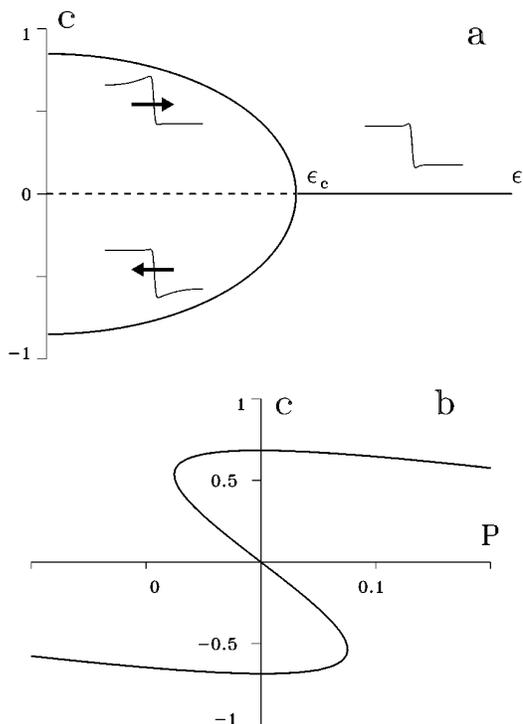
FIG. 1. Bifurcation diagrams for fronts in the bistable FHN reaction-diffusion system. (a) At the Nonequilibrium Ising-Bloch bifurcation a stationary front becomes unstable to a pair of counter-propagating fronts as a control parameter  $\epsilon$  is varied. The solid lines represent a branch of front solutions with speed  $c$ . (b) Unfolding the bifurcation near the critical point  $\epsilon_c$  gives an S-shaped relation in the unfolding parameter  $P$ .
