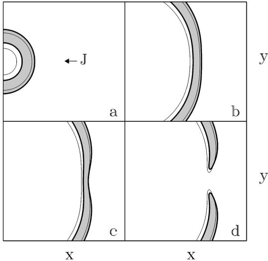
FIG. 5. Numerical solution of Eqs. (11) with a weak advective field  $\mathbf{J} = J\hat{\mathbf{x}}$ . The thick and thin lines pertain to  $u=0$  and  $v=0$  contour lines, respectively. The initial circular pulse fails to propagate along the direction of the advective field and the pulse breaks. The pulse continues to propagate in directions different from the advective field. The equation parameters are the same as in Fig. 4.
