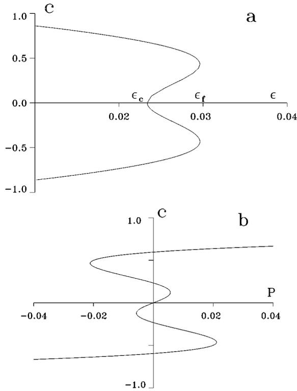
FIG. 2. Bifurcation diagrams for pulse solutions in the excitable FHN system. (a) A typical relation for the pulse speed  $c$  vs the system parameter  $\epsilon$  gives a subcritical pitchfork bifurcation. (b) Unfolding the bifurcation near the critical point  $\epsilon_c$  gives a multiple S-shaped curve for  $c$  in the unfolding parameter  $P$ .
