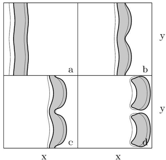
FIG. 7. Breakup of a pulse by transverse instability. The thick and thin lines pertain to  $u=0$  and  $v=0$  contour lines, respectively. The initial almost planar pulse is unstable to transverse perturbations and forms a dent. The dent grows and the pulse breaks at the region of high curvature. The equation parameters are the same as in Fig. 6.
