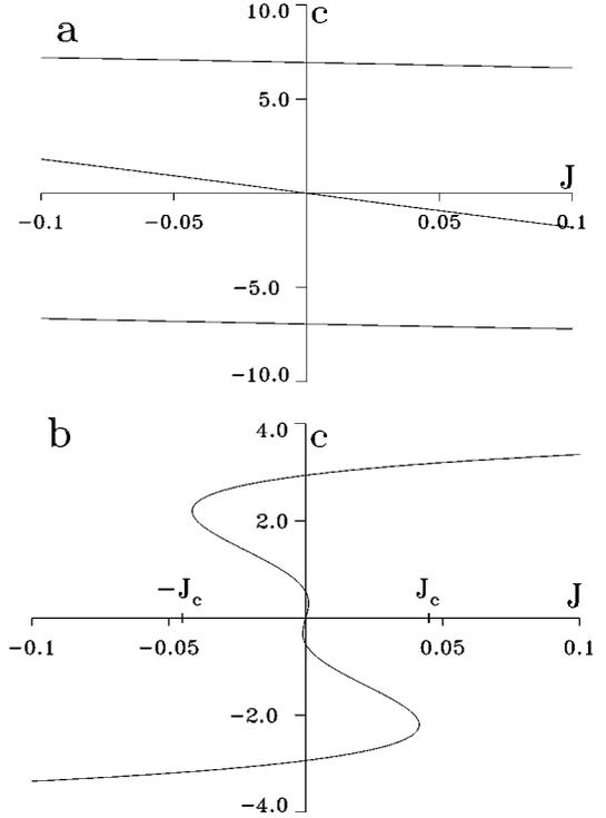
FIG. 4. Solutions of the speed  $c$  vs advection  $J$  relation (12). (a) Away from the bifurcation point, variations in  $J$  have little effect on the pulse speed ( $\epsilon=0.01$ ). (b) Near the bifurcation point, small variations in  $J$  may drive the system past the end point of the solution branch and cause pulse collapse ( $\epsilon=0.05$ ). Other parameters are  $a_1=1.25$ ,  $a_0=-0.2$ , and  $\delta=1.0$ .
