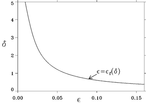
FIG. 3. Pulse failure propagation boundary in the  $\epsilon$ - $\delta$  parameter plane for the excitable FHN model. To the right of the line pulses fail to propagate. The parameters are  $a_1=1.25$  and  $a_0=-0.2$ .
