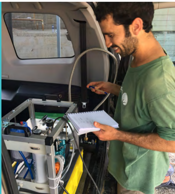
Dr. Roi Ram checking how the groundwater flows into a degassing device, Autumn 2018
