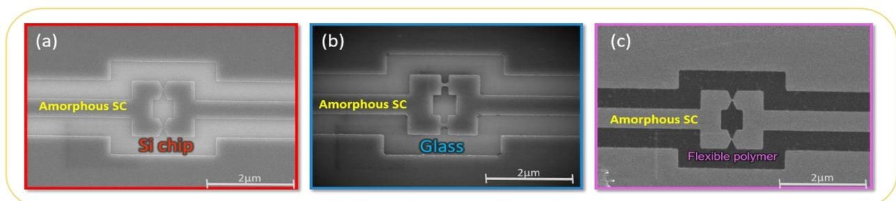
**Figure 1| Devices made of amorphous superconducting coatings on various substrates.** Electron micrographs of nanoscale amorphous superconducting quantum interference devices (SQUIDs) that are fabricated on (a) a SiO/Si chip, (b) a transparent glass substrate, and (c) an adhesive flexible polymer.
