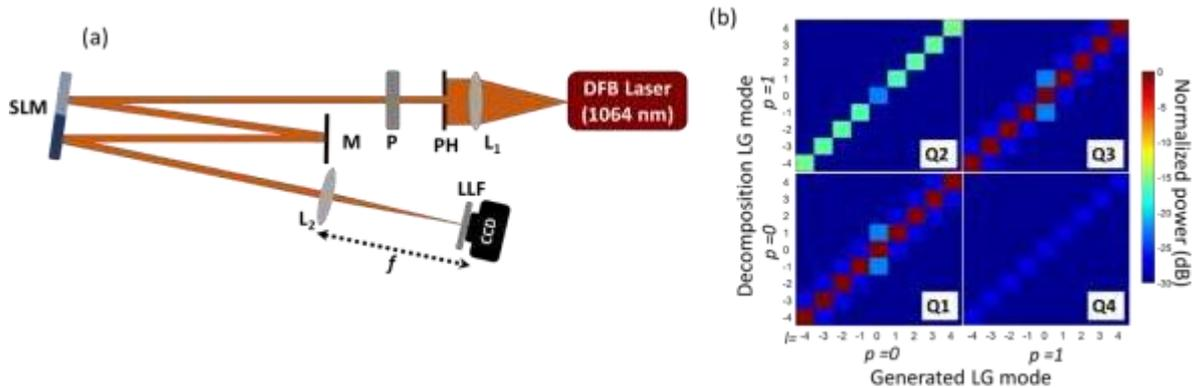
experimentally [4], we use a spatial light modulator (SLM) and convex lens as shown in Fig. 1(a).
