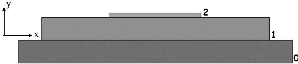
Figure 3. The DDA block system which constrains Block 2 to one degree of freedom – horizontal sliding only. Block 0 is the foundation block, Block 1 receives the dynamic input motion (horizontal – cyclic), and Block 2 responds.
