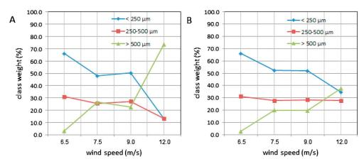
Figure 2. Sand fraction distribution at a sequence of wind speeds applied in the tunnel. Shown are sand collected from the two lower traps (a) T1 and (b) T2 at heights of 1 and 3 cm, respectively.
