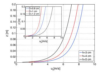
**Figure 4.** Threshold velocity for  $D_c = 1$  mm and  $u_a = 0.5$  m/s for ripples with different heights; z is the height above the surface. The inset shows the threshold velocity for different values of grain diameter (the other parameters are the same).
