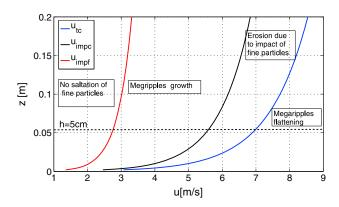
Figure 5. The different processes in megaripples evolution dictated by wind velocity at different height above the surface (Z). Parameters: h=5 cm, L=0.2 cm, D=1 mm, and  $u_{_{\ast}}=0.5$  m/s.
