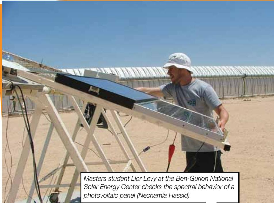
Masters student Lior Levy at the Ben-Gurion National Solar Energy Center checks the spectral behavior of a photovoltaic panel (Nechamia Hassid)
