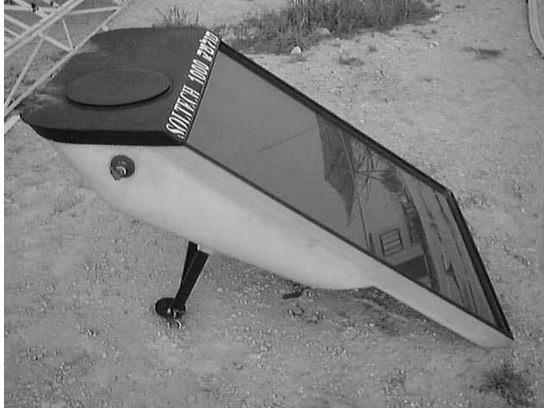
Fig. 1. The SOLTECH 1000™ integrated collector–storage solar water heater under study.
