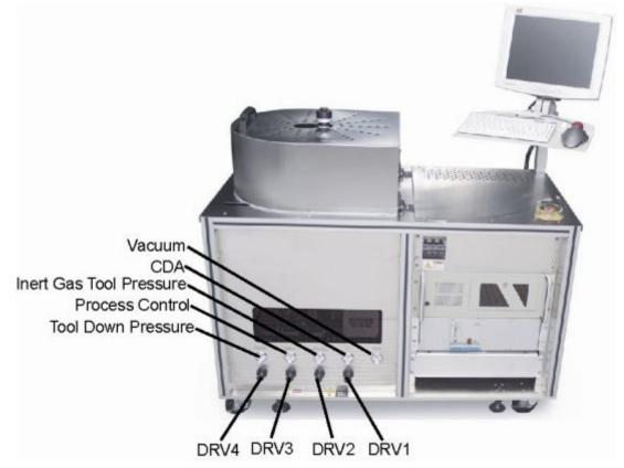
Figure 4-10 Pressure Gauges and Regulators
