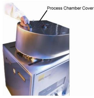
**Figure 6-1 Process Chamber Cover**
