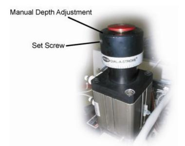
Figure 5-20 Location of Pressure Head Adjuster Set Screw
