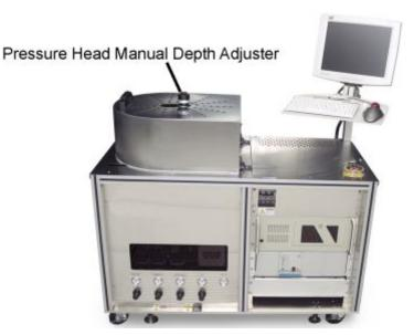
Figure 5-19 Location of Pressure Head Manual Depth Adjuster
