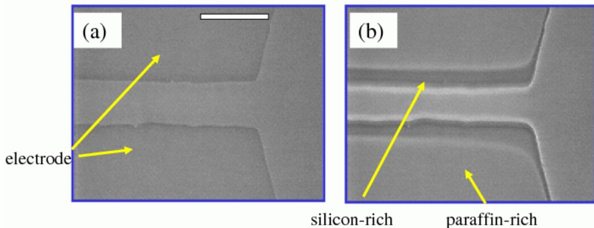
Field-induced phase transition in mixtures of simple liquids. (a) Field off. Two flat electrodes are covered with homogeneous mixture of silicon oil and paraffin. (b) Field on. Silicon-rich domains form close to the electrodes' edges, paraffin-rich phase is elsewhere. Bar is 50  $\mu\text{m}$  [*Nature* **430**, 544 (2004)].
