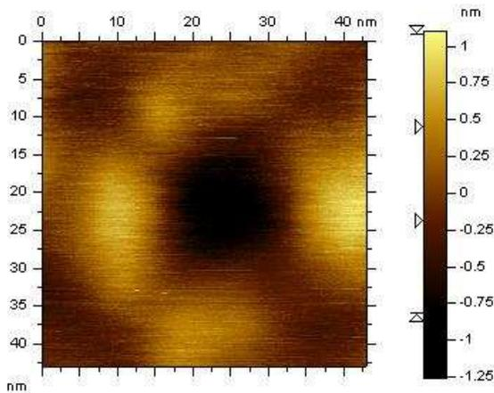
**High-resolution AFM topography image of the surface of a hybrid photovoltaic film**
