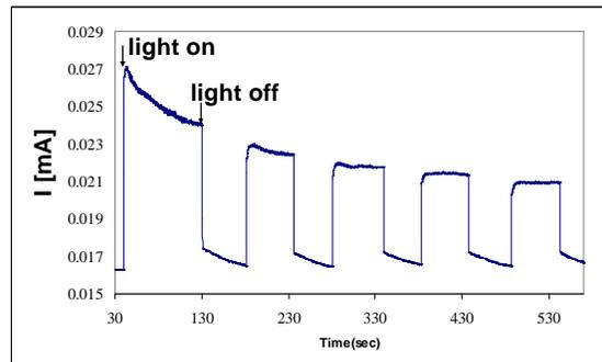
**Photovoltaic current in nano-structured photoelectrochemical cell**
