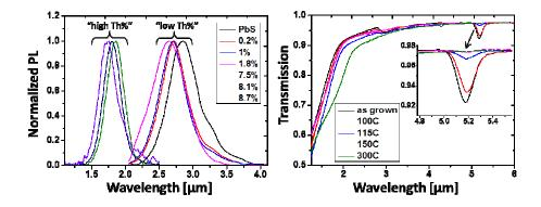
The optical properties of PbS thin films alloyed with thorium and oxygen, were characterized by the vertex 80v. Those thin films are highly important in the technology of infrared detectors.
