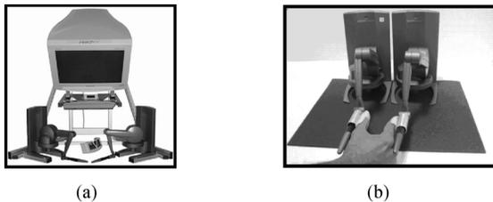
Fig. 1. The virtual reality system. (a) The dual Reachin/Sensegraphics display system is based on two robotics devices and an augmented reality display that allows subjects to see and feel objects with both hands within a small workspace. (b) One thimble connects the index finger and another thumb to a robotic arm.
