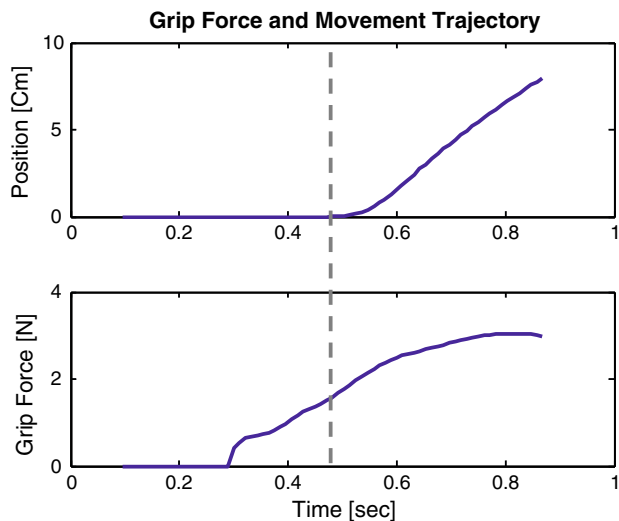
Fig. 4 Single trajectory movement and GF records from one subject lifting a load of 300 g. Dashed vertical line indicates the onset time of the movement using the MACC-based algorithm
